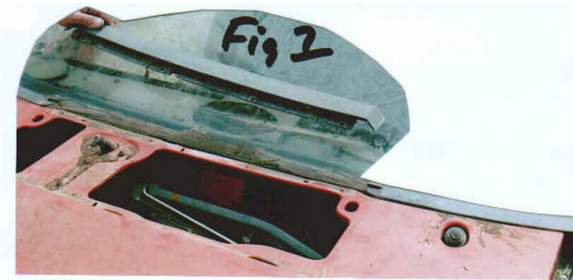
1. Remove existing cowl vent cover and trim strip in center of windshield.
